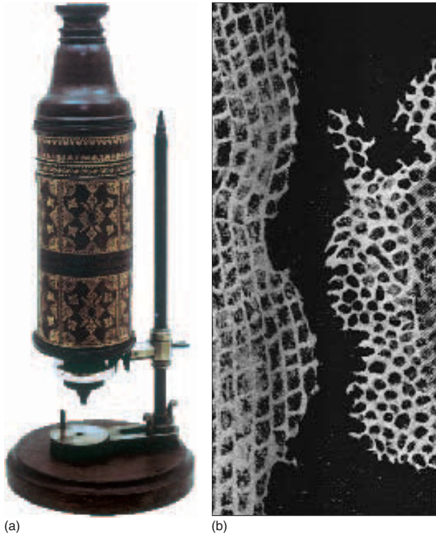
Figure 1.5 Hooke's Compound Microscope. (a) The compound microscope had a lens at each end of a tubular body. (b) Hooke's drawing of cork cells, showing the thick cell walls characteristic of plants.
